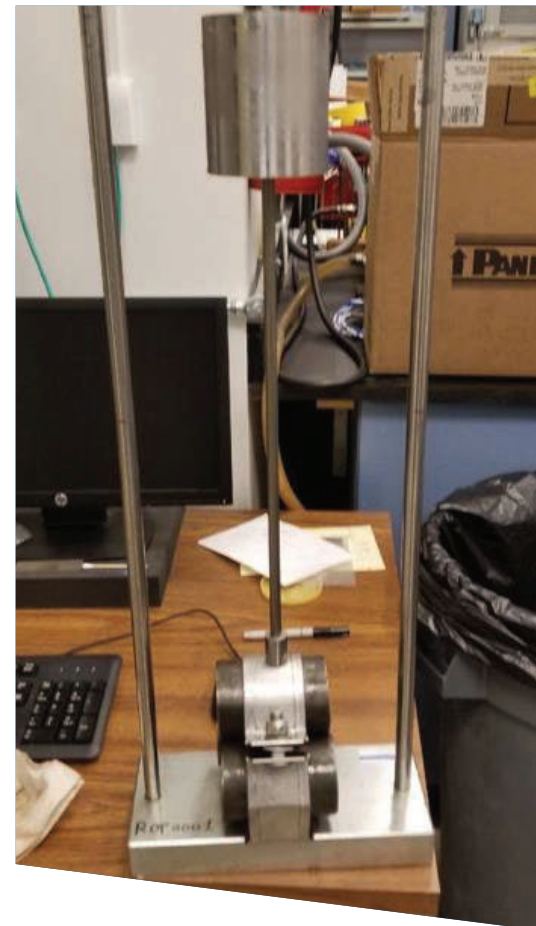
Fig 10: Testing of Impact Resistance Test- Panduit Lab Test Setup
