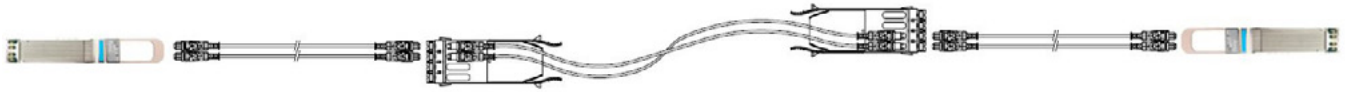
View is 'top view' of link. MPO's will be installed vertically on 800G dual MPO transceivers
