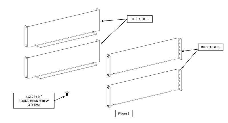
• The 2-Post Rack-Mount Adapter Kit consist (2) LH and brackets, (2) RH brackets and  $(24) #12-24 x \frac{1}{2}$  round head screws.
