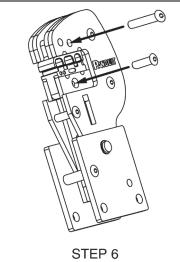
Step 7: Die halves should align front and back; and side-to-side.
