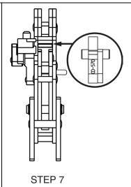
Re-insert Crimp Head with newly installed Crimp Die Inserts into the tool per the instructions on Page 1.
