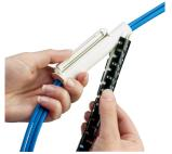
Slide Pan-Wrap™ Split Harness Wrap onto end of tool until approximately 3" of it covers the bundle.
