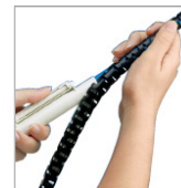
Grasp end of Pan-Wrap™ Split Harness Wrap and bundle while pulling the tool along the bundle length.
