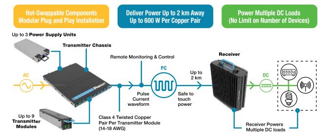
Overview of the FMPS, showing the Transmitter Chassis which typically resides in the headend, delivering power in a Pulse Current waveform, through multi-conductor Class 4 cable, and sending it to the FMPS Receiver which is typically distributed throughout the building near devices that require power.
